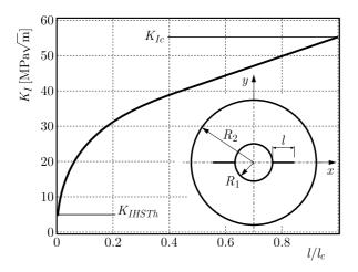
Fig. 5. The dependence of the stress intensity factor on the relative length of the crack, and a scheme of the disk with two cracks
