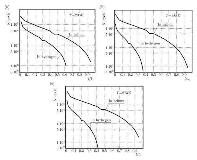
Fig. 7. Dependence of the number of cycles to fracture on relative length of the crack (in helium – solid line, in hydrogen – dashed line) for different temperatures: (a) T = 293 K, (b) T = 483 K, (c) T = 673 K
