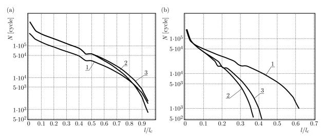
Fig. 6. Dependence of the amount of cycles to destruction from relative length of the crack in helium (a) and in hydrogen (b) for different temperatures: 1 - T = 293 K, 2 - T = 483 K, 3 - T = 693 K
