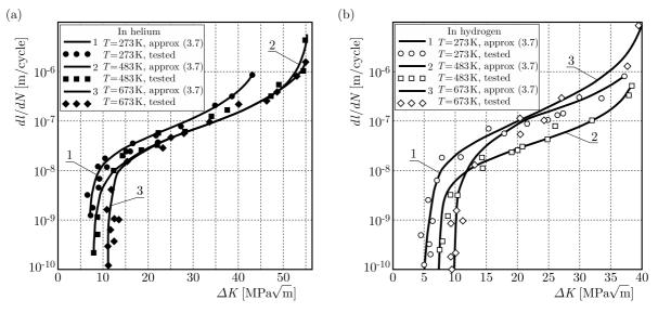
Fig. 4. Kinetic fatigue fracture diagrams of steel 10Kh15N27T3V2MR in helium (a) and in hydrogen (b) at different temperatures: 1 - T = 293 K, 2 - T = 483 K, 3 - T = 673 K (curves are approximations from formulas (3.7) and (3.8), symbols are experimental data)
