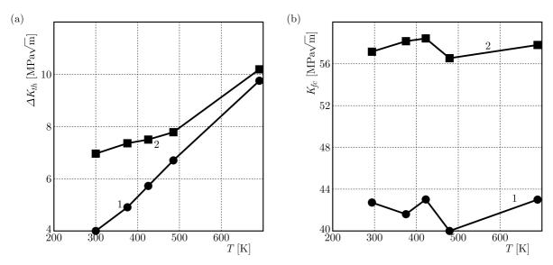
Fig. 3. Influence of temperature on the parameters of cyclic crack resistance  $\Delta K_{th}$  (a) and  $K_{fc}$  (b) in helium (2) and in hydrogen (1) pressure 30 MPa after prehydrogenation (623 K, 30 MPa, H2, 10 h)
