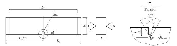
Fig. 1. Beam sample for research on cyclic crack resistance
